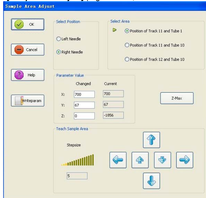
Fig. 1.7.2-1: [Sample Area Adjust] (Right Needle, Position of Track 11 and Tube 1)
