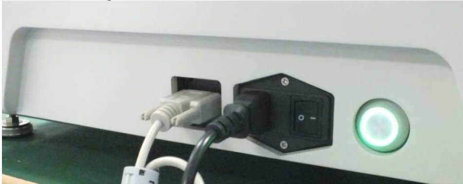
Fig. 3.2.13-1: Electrical and electronic connections.
