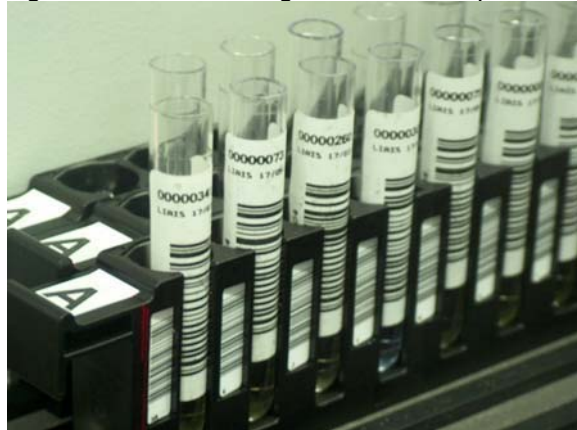
Fig. 15.3.1.5-1: Inserting bar-coded sample tubes
