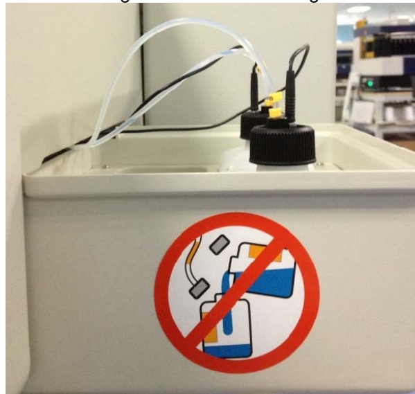
Fig. 3.2.10-1: Starter reagent container on the right side of the analyzer.
