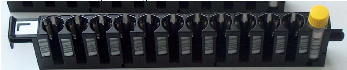
Fig 13.2.4-1: Light Check inserted in an rack
