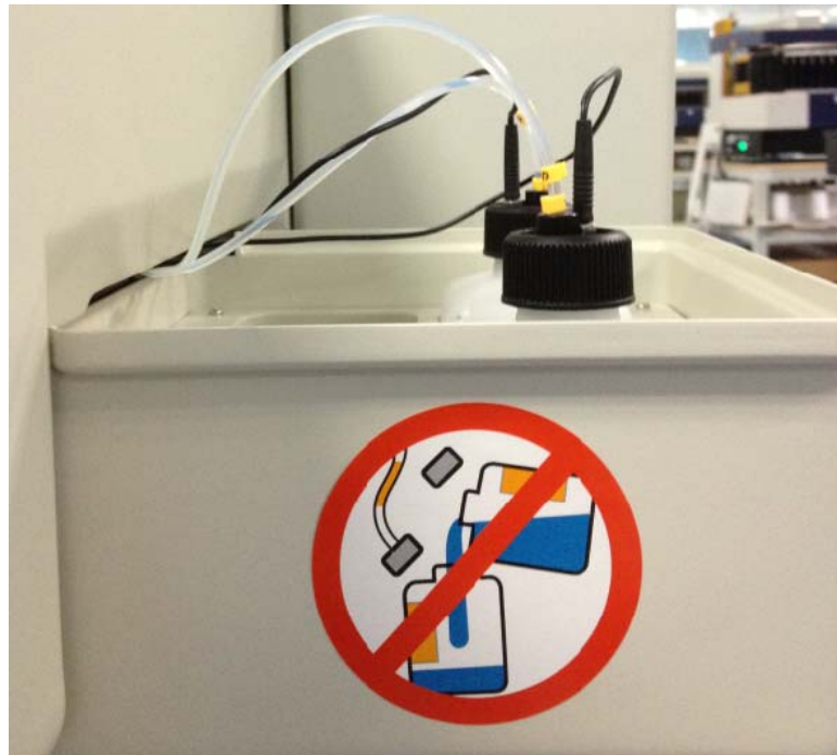
Fig. 8.3-1: No-Pooling Warning Labels on Starter Reagent housing
