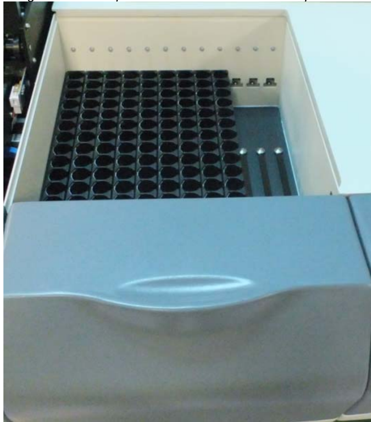
Fig. 3.2.1-2: Sample station with 12 tracks for sample racks.
