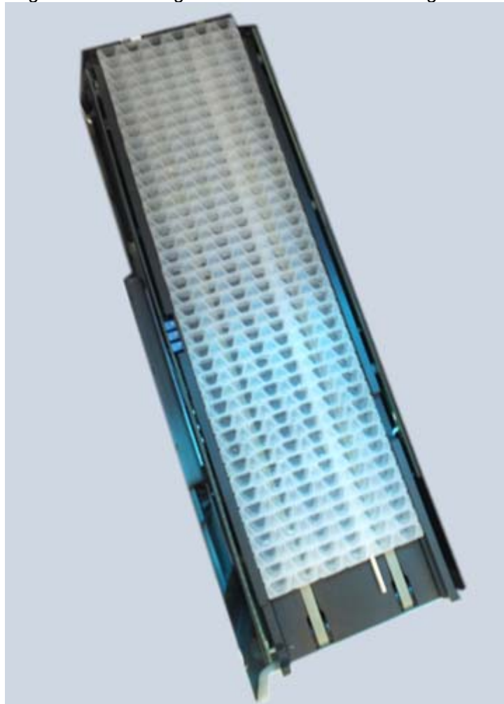
Fig. 3.2.8-1: Loading with reaction modules on Maglumi 800
