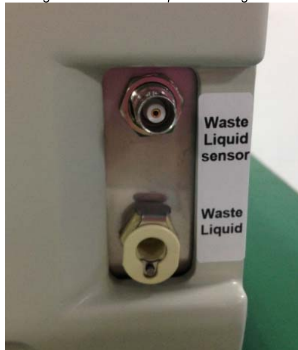
Fig. 3.2.10-1: drainage tubes for waste liquid on the right side of the analyzer.
