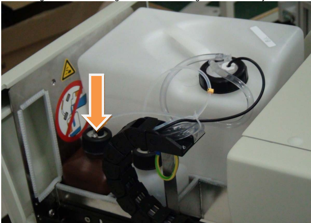
Fig. 3.2.9-1: Starter reagent container on the right side of the analyzer.
