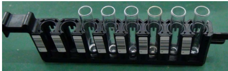
Fig. 3.2.1-1: An example of the sample rack for 8 samples
