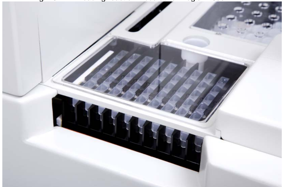
Fig. 13.2.1-1: loading reaction modules for Maglumi 600.
