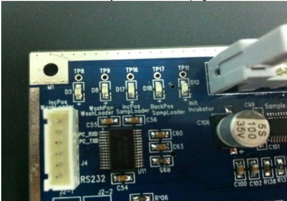
Fig. 1.2.2-3: MAGLUMI600 analyzer master board 03program download interface: J4
