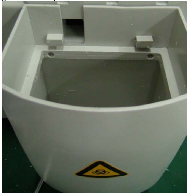
Fig. 3.2.11-1: Disposal of reaction modules
