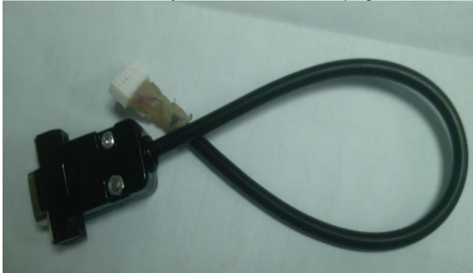
Fig. 1.2.2-1: MAGLUMI600 analyzer master board 02-04, program download line
