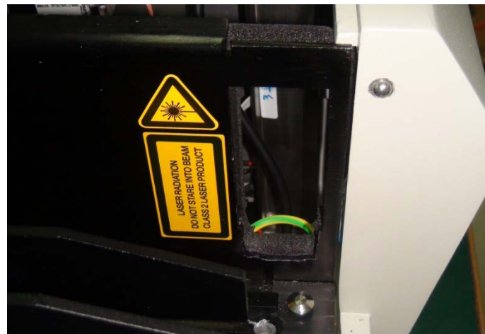
Fig. 8.2-1 Laser Beam Warning at the Sample Loading Area
