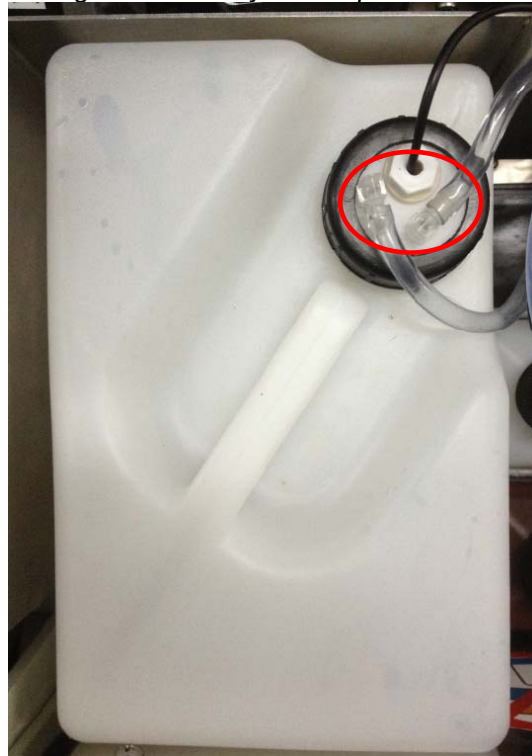
Fig. 13.2.2.1-1 System Liquid connections.
